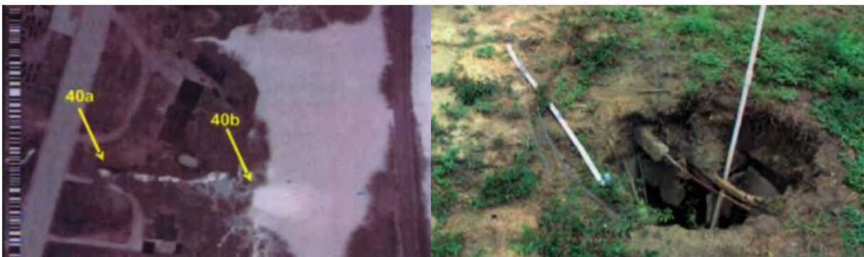
Figure 6-7: Infrared thermographic image showing septic illicit discharge (left) and the discovered cave-in responsible for the problem (Source: US EPA, 2016)
